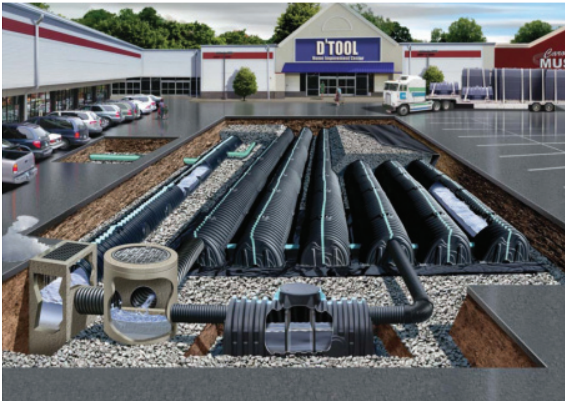
Schematic of the CULTEC Stormwater Chamber (Image source: CULTECH).
