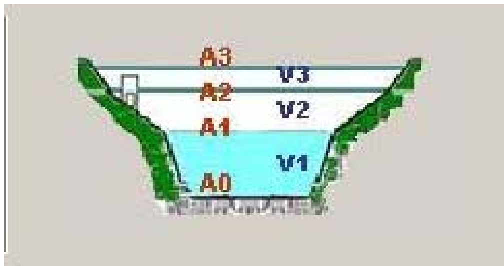
Figure 4-34. The BMPDSS multi-stage pond module.
